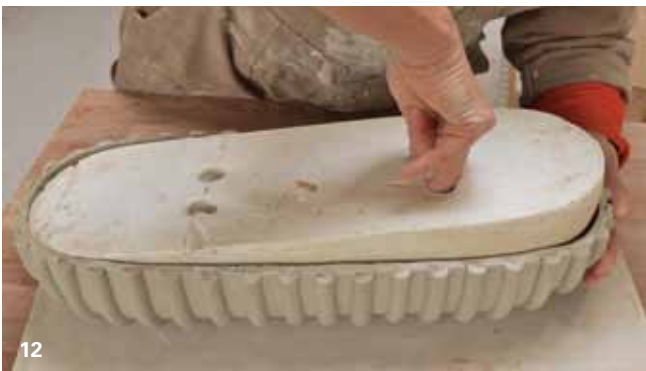
12 Loosen the edge of the rim slightly from the plaster to enable the mold to be lifted up and separated from the clay form.
