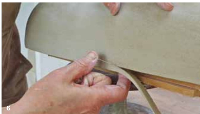
6 Use a wire tool to cut off any excess clay along the edge to make the rim level, then smooth the edge.
