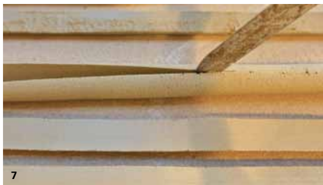
7 Extrude long, even coils and split each coil precisely in two halves with a knife.
