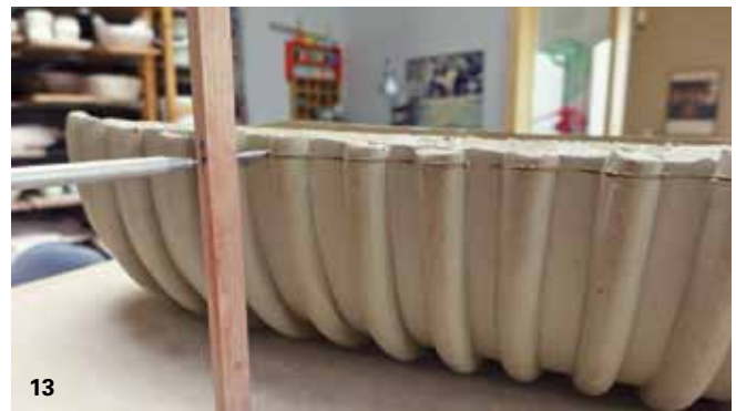
13 Make a horizontal line around the bowl with a needle tool fitted into a square board. Cut off the rim with a sharp knife.
