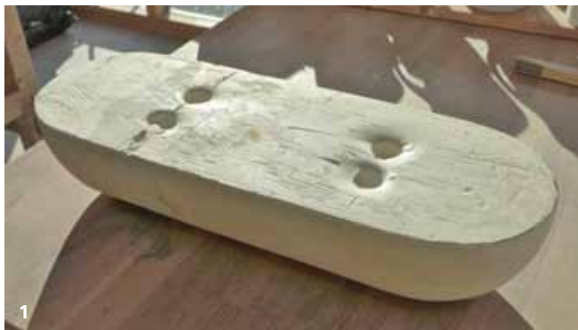
1 Plaster hump mold with angled finger holes to pull the mold up and out of the clay form.
