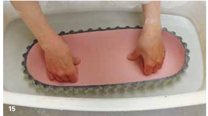
After glazing the interior, push the bowl down in to a vat of glaze up to the rim to coat the exterior.
